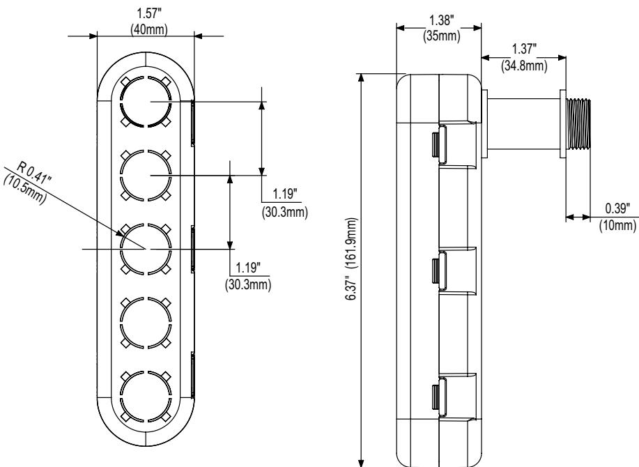
The extender module snaps apart to allow wires to thread through it and into the fixture for connection. It then snaps together to protect wires.
