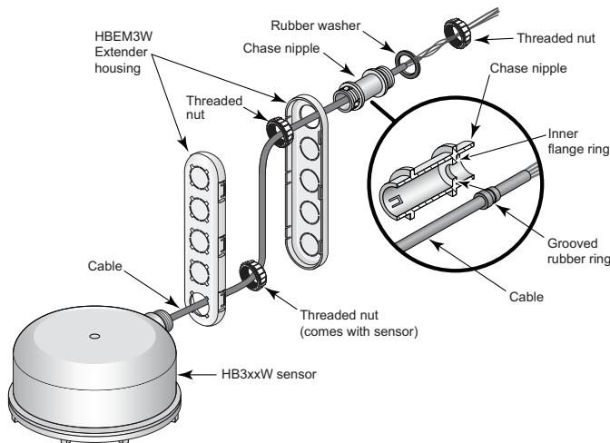
The chase nipple snaps into the extender housing, while the other end fits into a watertight fixture enclosure with a standard knockout. A rubber washer fits between the nipple's outside flange and the outside of the fixture. Use the included nut to secure the nipple and rubber washer against the inside wall of the fixture enclosure.
