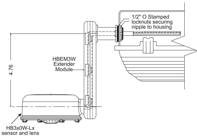
Snap the extender module apart to thread the wiring cable through it and into the fixture for connection.
