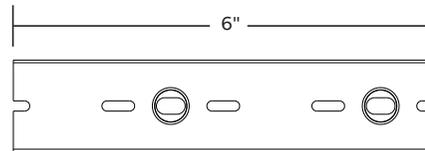
Minimum mounting rivet distance for ducts 1.5" wide.
