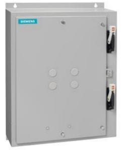
Duplex starter with alternator Size 3 1/2 Three phase full voltage Amb compensate bimetal OLrelay Contactor amp rating 115Amp 110VAC 50HZ / 120VAC 60HZ coil Combination type Two 200A disconnect switches Encl NEMA type 4 painted steel Water/dust tight non-corrosive
