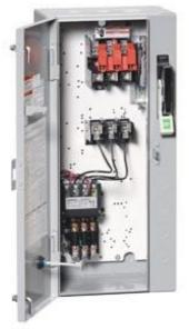
Non-reversing motor starter Size 2 Three phase full voltage Amb compensate bimetal OLrelay Contactor amp rating 45Amp 240VAC 50HZ / 277VAC 60HZ coil Combination type 60Amp fusible disconnect 60Amp / 600V fuse clip Enclosure NEMA type 1 Indoor general purpose use Standard width enclosure
