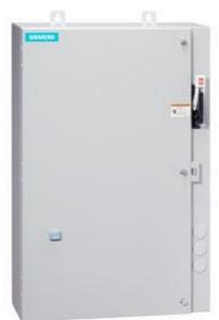
Non-reversing motor starter Size 4 Three phase full voltage Solidstate overload relay OLRelay amp range 50-200A 110V 50HZ / 120V 60HZ coil Combination type 150A circuit breaker Enclosure NEMA type 4/12 Water/dust tight for outdoors Standard width enclosure
