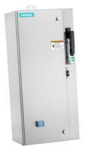
Non-reversing motor starter Size 1 Three phase full voltage Solidstate overload relay OLRelay amp range 0.25-1A 220-240/440-480VAC 60HZ coil Combination type 30Amp fusible disconnect 30Amp / 250V fuse clip Encl NEMA type 4X 304 S-steel Water/dust tight non-corrosive Standard width enclosure
