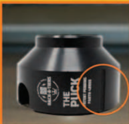
An "indicating line" for use when working blind.
