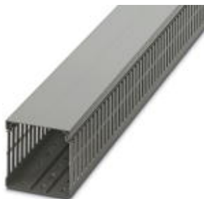
Cable duct, gray, consisting of upper and lower part, width: 80 mm, height: 80 mm, length 2000 mm
