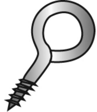
*These screw eyes are bolts with a formed closed circular eye fashioned at the non-threaded end and lag threaded screws on the other.*
