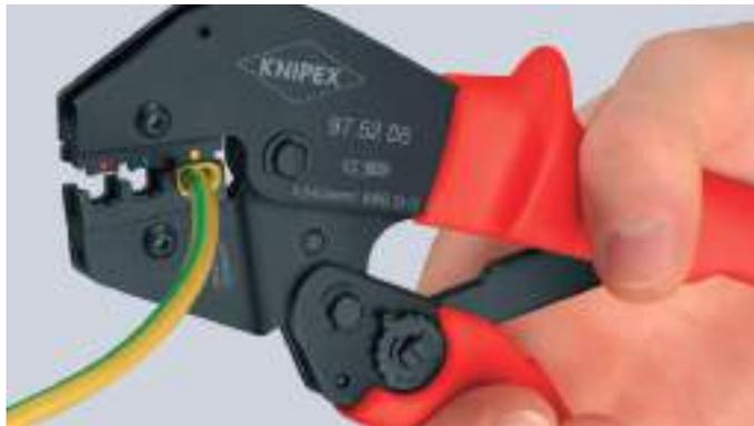
Second step: insert wire into connector and squeeze handles to complete crimp
