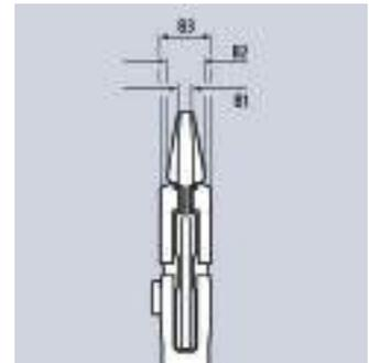
Open end wrenches with fixed opening widths are expensive, especially when used for large union joints. The KNIPEX Pliers Wrench XL, with its adjustable jaw opening up to AF 3 3/8" (85 mm), offers enormous savings potential.
