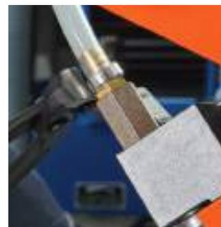
Sealing the hose connection on central lubrication
