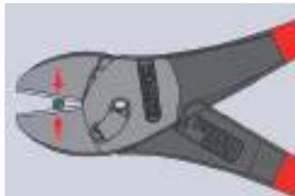
Insert the wires as close to the hinge as possible. In case of cutters with very high transmission, the width of the gap between the cutting edges close to the fulcrum may be less than the thickness of the wire. Wires may slip forward when the cutting starts.
