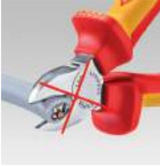
Cut performed with a Diagonal Cutter: high effort required, inaccurate cut, considerable deforming and crushing of the cable.
