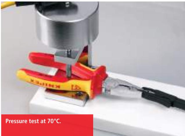
Pressure test at 70°C.
