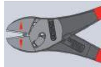
First make a notch in the wire using the KNIPEX TwinForce® until the required hand force increases considerably. Now open the pliers and slide the wire backwards towards the joint.
