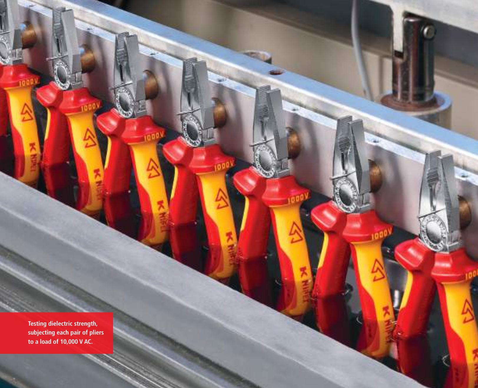
Testing dielectric strength, subjecting each pair of pliers to a load of 10,000 V AC.
