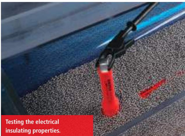
Testing the electrical insulating properties.
