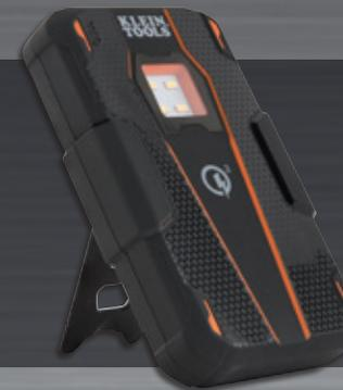
The **KTB2** features a 170-lumen work light and multi-position kick stand. It is equipped with class-leading, fast-charging capabilities on all of its ports, which include Type-A Qualcomm® Quick Charge™ Technology, USB Type-A (2.4A) and USB Type-C (3.0A).
