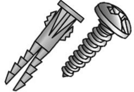
*An injection-molded anchor with a ribbed shank which resist "backing-out" after installation and longitudinal slits along the shaft which allows the anchor to expand when a screw is inserted.*
