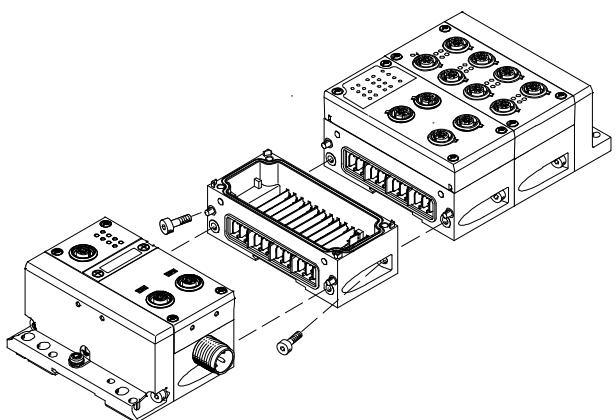
The CPX modules are mechanically connected using a special angled fitting. The CPX terminal can thus be expanded at any time.
