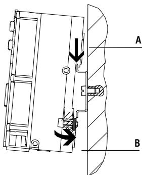
The H-rail mounting is part of the reverse profile of the CPX interlinking blocks. The CPX terminal can be attached to the H-rail using the H-rail mounting kit. The CPX terminal is mounted on the H-rail for this purpose (see arrow A).
