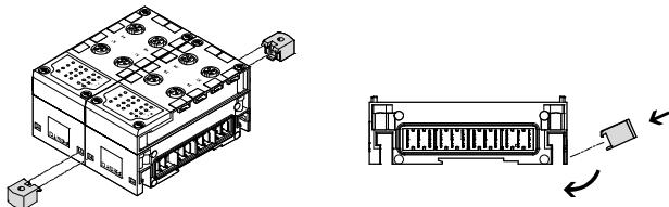
For longer valve terminals, there are additional mounting components for the CPX terminal that can be fitted between two modules.
