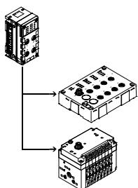
The electrical interface CPX-CTEL-2... enables the connection of modules with IO-Link interface (IO-Link device) to the CPX terminal. The I/O data of the connected devices are transmitted to the connected CPX bus node and thus to the higher-order controller via fieldbus.
