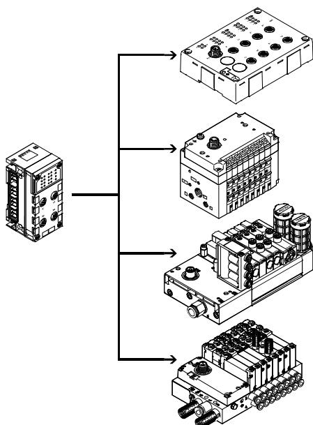
The CPX-CTEL master provides four I-Port interfaces to which one device each can be connected. I-Port is an interface for exchanging serial data for connecting decentralised modules or valve terminals from Festo. The I-Port interface is based on IO-Link and is compatible with it in certain areas. The connection type corresponds to a star topology. In other words, only one module or valve terminal can be connected to each I-Port.
