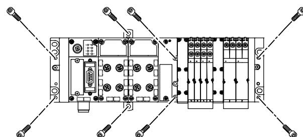
The end plates of the CPX terminal, the valve terminal and the pneumatic interface include mounting holes for wall mounting. Additional mountings for the CPX terminal are available for longer valve terminals. These mountings differ depending on the design of the CPX terminal (plastic or metal).
