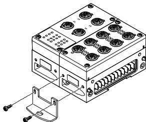
For longer valve terminals, there are additional mounting brackets for the CPX terminal that can be screwed onto the interlinking blocks. The mounting bracket CPX-M-BG-VT-2X enables a CPX terminal with valve terminal VTSA/VTSA-F to be mounted on a support system.
