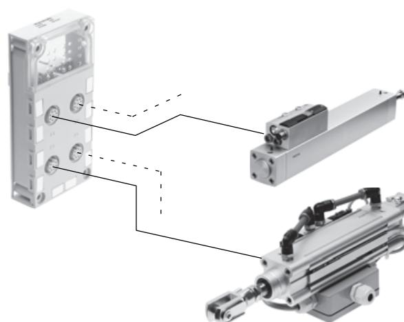
Since the module supports the M12 connection block (8-pin), up to 4 cylinder/valve combinations with integrated sensors can be connected. Each cylinder/valve combination is supported by 2 inputs and 2 outputs per connection. It is therefore possible to control max. 2 solenoid coils and record signals from 2 sensors with a pre-assembled connecting cable.
