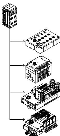
The electrical interface CPX-CTEL master establishes the connection to modules with I-Port interface (device) from the CTEL/CTEU series. The I/O data from the connected devices is transferred to the connected CPX bus node and therefore transferred to the higher-level controller via fieldbus. A maximum of 4 devices can be connected to a CPX-CTEL master via appropriate M12- interfaces.
