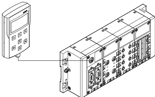
The operator unit is connected to the CPX terminal using a pre-assembled connecting cable.
