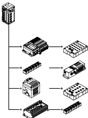
The CPX-CP electrical interface establishes the connection to CP modules of the CPI installation system via prefabricated connecting cables. The I/O data of the connected valve terminals with CP string extension and CP input and output modules are transferred to the connected CPX bus node and thus via fieldbus to the higher-order controller. This enables modular centralised and compact decentralised concepts to be established with one system.
