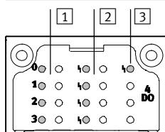
1 Status LEDs for the inputs and outputs
