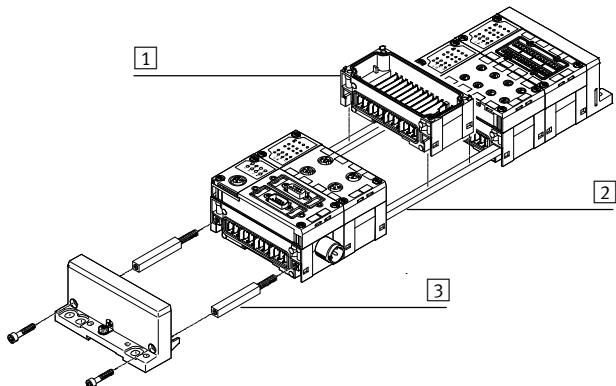
The CPX modules are mechanically connected using special tie rods [2]. Two screws in the end plates are all that are needed to assemble the entire unit. The tie rod ensures that the unit resists high mechanical loads and is therefore the mechanical backbone of the CPX terminal.
