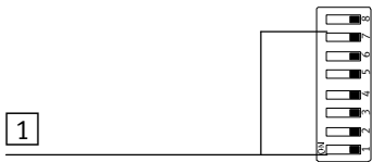
Fig. 1/4: Setting the station number (8-element DIL switch 3)
