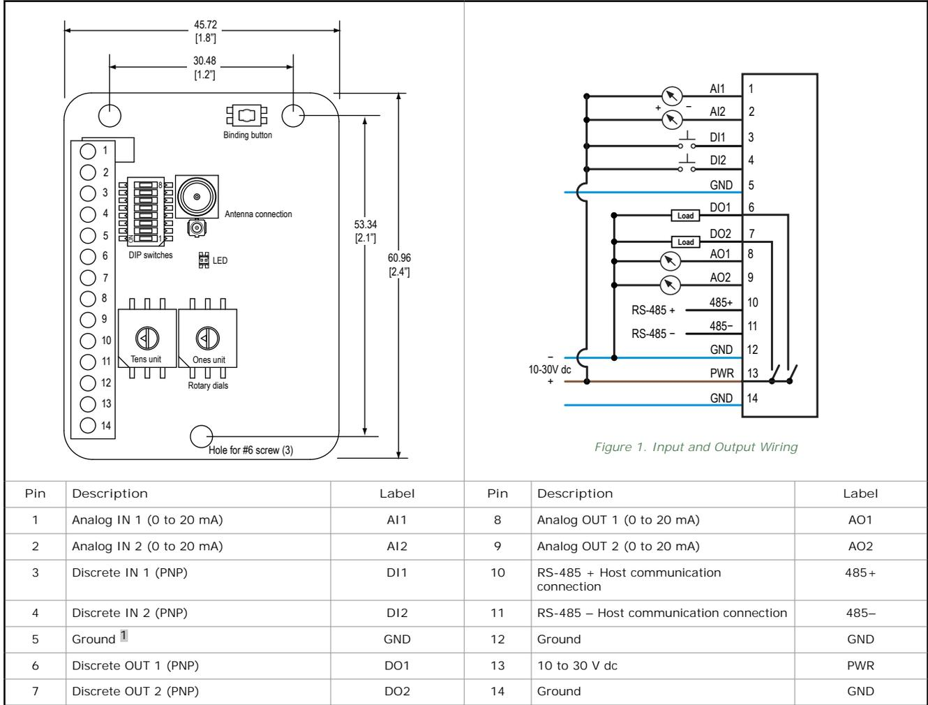
Figure 1. Input and Output Wiring
