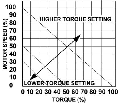
In the NL position, only torque (not speed) is varied by the input signal. The motor output torque remains constant over the motor's full speed range unless the load is less than the set torque. If the load torque decreases below the set torque, the motor will rapidly increase to full speed. This type of torque control is applicable to processes where the torque must remain constant over a wide motor speed range. The NL torque characteristics are shown in Figure 2-14.
