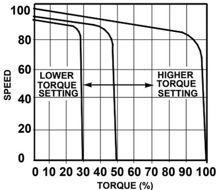
Because the BC200/BC201TM are regenerative controls, torque will be applied in both forward and reverse directions. The maximum torque can be set with the FWD CL and REV CL trim pots, and by using the FWD ACC and REV ACC trim pots, the rate of change of torque can be made more or less gradual. The maximum speed trim pot can be used to set the maximum motor speed under a no load condition.
