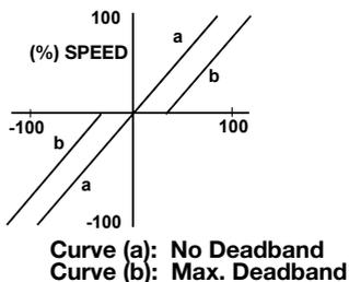
Note: If the deadband trimpot is set too low (CCW direction), the motor may oscillate between forward and reverse. Adjust deadband trimpot CW until the instability disappears. (Oscillation may also occur due to response setting.)
