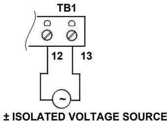
Note: Terminal 13 is common. A positive signal with respect to terminal 13 will produce a positive output to motor. A negative signal with respect to terminal 13 will produce a negative output. A 0 to  $\pm 10$  VDC is required to operate control from 0 to  $\pm$  full output. If required, use the (Optional) BC212, Signal Isolator.
