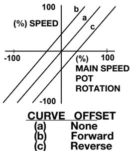
**Figure 2-12 Deadband Trimpot Adjustment**
